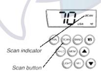
Pressing the SCAN button again will disengage scan.
