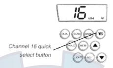
Channel 16 represents the same frequency on both USA and INT bands. If 16 is pressed again, the DC5s will return to the previously selected channel.
