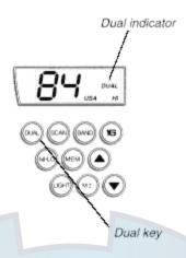
Select any channel on either USA or INT bands. Press DUAL. The DC5s will monitor your selected channel and channel 16 simultaneously. If a transmission is heard on either channel, that channel will continue to be selected until no further transmission is received, then dual watch will be re-engaged.
